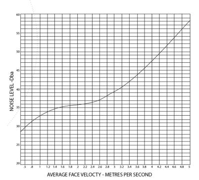
Curve corrected for background noise level at 1Db less than measured noise level. For background noise levels below figures from this graph, reduce graph figures by amounts listed in following table. Background noise level would comprise Duct Air Borne Noise, Damper Noise, etc.
